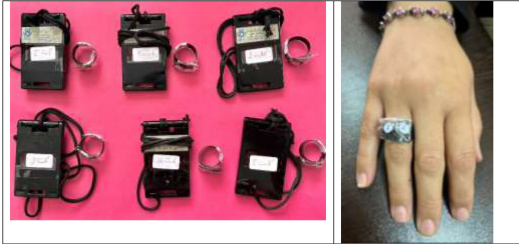
Fig. 2. Rings and Cards for measuring Hp(0.07) and Hp (10) respectively.
