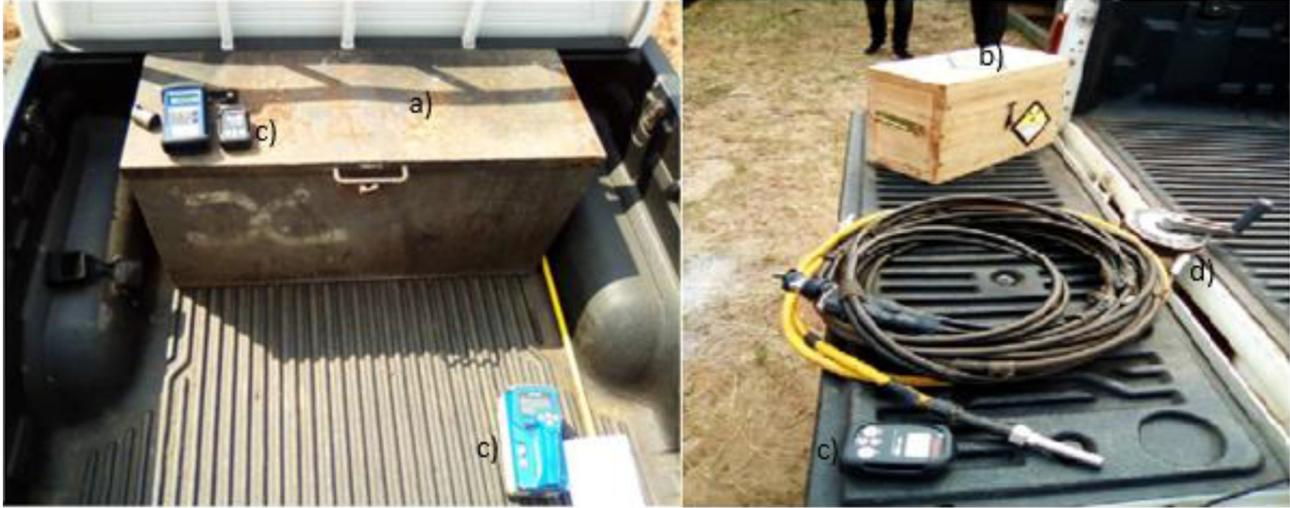
**Fig. 1.** The gamma radioactive source used during the evaluation. Here the source is either within a fixed box on the transport vehicle (a) or within a simple transportation box (b). Are also shown the survey meters used to measure ambient dose equivalent rates (c) and the accessories (d)–remote control, ejection cable and guide tube–for exposing the sealed gamma source.
