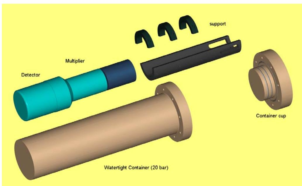
**Figure 1.** The watertight cylindrical enclosure, which houses the sensor, the photomultiplier and the appropriate sled.
