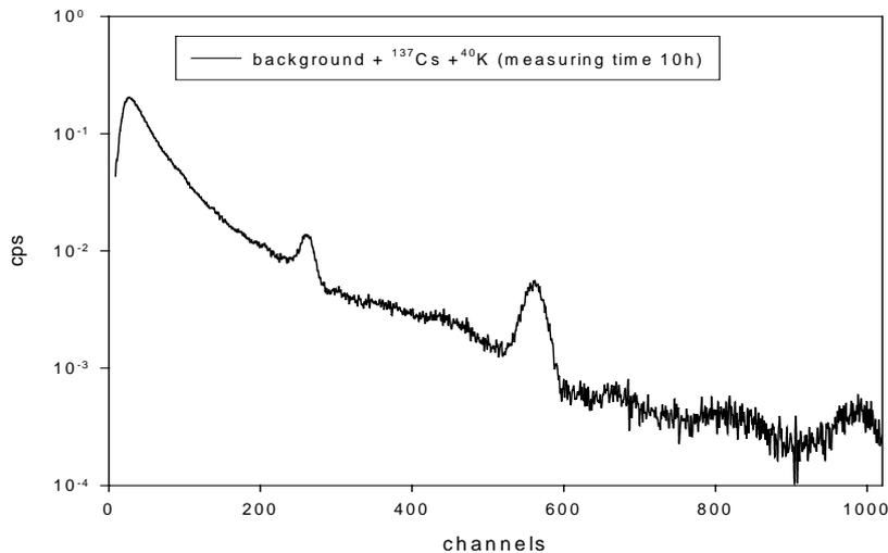
**Figure 3.** The acquired spectrum with the calibration reference sources:  $^{40}\text{K}$  and  $^{137}\text{Cs}$ .
