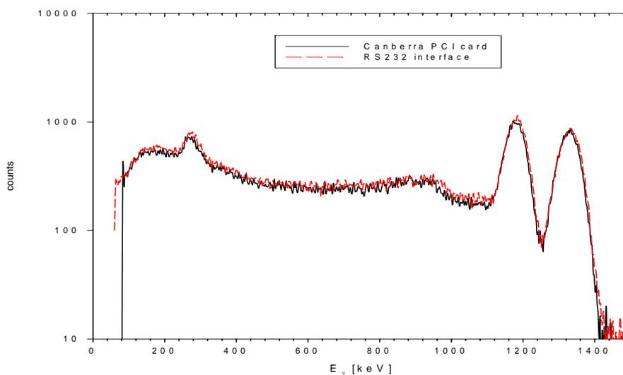
**Figure 2.** The measured spectra as acquired by the Canberra PCI card as well as by the developed electronics with RS232 communication. The two measurements were performed in the same geometry by using the  $^{60}\text{Co}$  reference source and the measuring time was 100 s.
