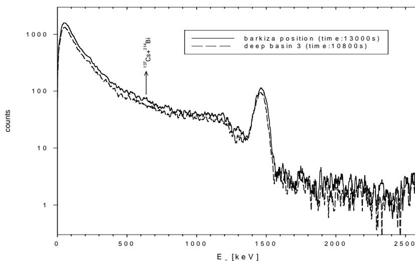
**Figure 4.** The measured spectrum at the DB3 (3m) and at Varkiza (Athens) position in a depth of 3m. The measuring times are 10800 and 13000 seconds respectively. The measured spectrum in Varkiza is after a rainfall.
